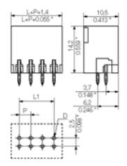
1728840000 S2L 3.5/16/180G3.5SN OR PCB plug-in connector, Male connectors, Soldered connection, Pitch: 3.50 mm, No. of poles: 16, 180°, Box 4032248036882 50 pc(s).
