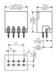
1728810000 S2L 3.5/10/180G3.5SN OR PCB plug-in connector, Male connectors, Soldered connection, Pitch: 3.50 mm, No. of poles: 10, 180°, Box 4032248040261 50 pc(s).
