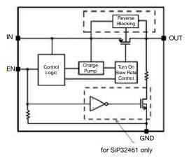
Fig. 2 - Functional Block Diagram
