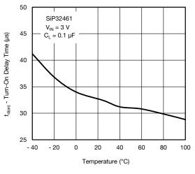
Fig. 15 - Turn-On Delay Time vs. Temperature
