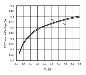
Fig. 16 - EN Threshold Voltage vs. Input Voltage
