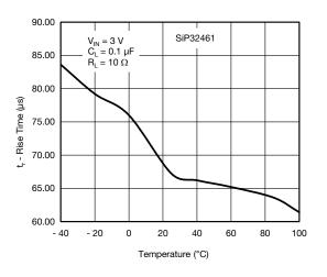
Fig. 17 - Rise Time vs. Temperature
