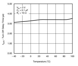
Fig. 20 - Turn-Off Delay Time vs. Temperature
