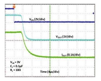
Fig. 22 - Turn-Off Time (V\_{IN} = 3 V, R\_L= 10  $\Omega, \ C_L$  = 0.10  $\mu F)$
