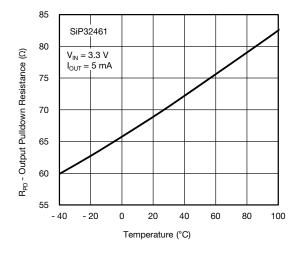
Fig. 19 - Output Pulldown Resistance vs. Temperature
