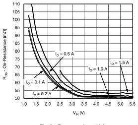
Fig. 9 - R<sub>DS(on)</sub> vs. Input Voltage
