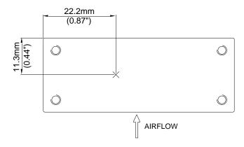
**Figure 23:** \* Hot spot temperature measured point, the allowed maximum hot spot temperature is defined at 102  $\mathcal C$
