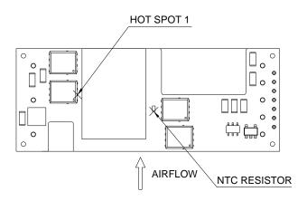
**Figure 21:** \* Hot spot 1 temperature measured point, the allowed maximum hot spot 1 temperature is defined at  $114^{\circ}C$
