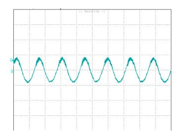
Figure 14: Output voltage ripple at nominal input voltage and rated load current (Io=20A)(50 mV/div, 2us/div)
