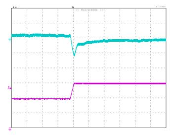
Figure 8: Output voltage response to step-change in load current (75%-50% of Io, max; di/dt = 0.1A/μs, Vin=48V). Load cap:220μF, electrolytic capacitor; 10μF, tantalum capacitor and 1μF ceramic capacitor. Top Trace: Vout (200mV/div, 200us/div); Bottom Trace: Io (10A/div, 200us/div). Scope measurement should be made using a BNC cable (length shorter than 20 inches). Position the load between 51 mm to 76 mm (2 inches to 3 inches) from the module..
