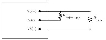
Figure 19: Circuit configuration for trim-up (increase output voltage)
