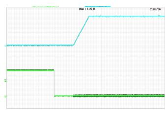
Figure 4: Turn-on transient at zero load current) (20ms/div). Top Trace: Vout; 5V/div; Bottom Trace: ON/OFF input: 5V/div.
