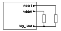
Corresponded to each octal digit, the requested resistor values are shown in below, and +/-1% resistors accuracy can be accepted. If there is any resistances exceeding the requested range, address 127 will be return. 0-12 and 40, 44, 45, and 55 in decimal address can't be used, since they are reserved according to the SMBus specifications, and which will also return address 127.
