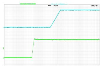
Figure 6: Turn-on transient at zero load current (20 ms/div). Top Trace: Vout; 5V/div; Bottom Trace: input voltage: 30V/div.
