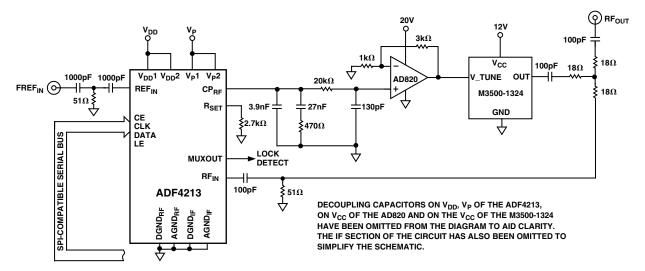
Figure 8. Wideband PLL Circuit
