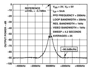
TPC 7. ADF4213 Reference Spurs (900 MHz, 200 kHz, 35 kHz)
