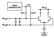
Figure 3. RF/IF Input Stage
