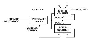
Figure 4. RF/IF A and B Counters
