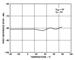
TPC 19. ADF4213 Reference Spurs vs. Temperature (836 MHz, 30 kHz, 3 kHz)
