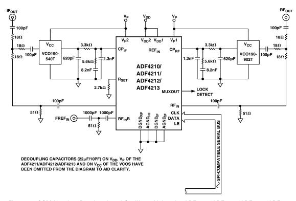
Figure 7. GSM Handset Receiver Local Oscillator Using the ADF4210/ADF4211/ADF4212/ADF4213
