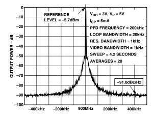
TPC 6. ADF4213 Reference Spurs (900 MHz, 200 kHz, 20 kHz)
