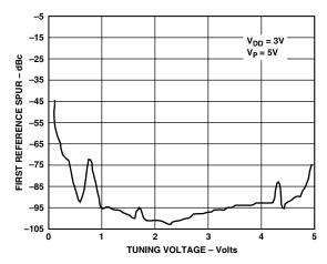
TPC 15. ADF4213 Reference Spurs (200 kHz) vs. V  $_{\rm TUNE}$  (900 MHz, 200 kHz, 20 kHz)
