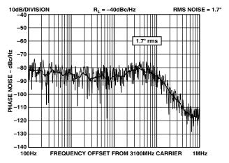
TPC 12. ADF4213 Integrated Phase Noise (2800 MHz, 1 MHz, 100 kHz)
