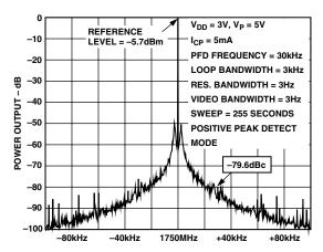
TPC 11. ADF4213 Reference Spurs (1750 MHz, 30 kHz, 3 kHz)
