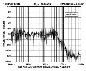
TPC 3. ADF4213 Integrated Phase Noise (900 MHz, 200 kHz, 35 kHz, Typical Lock Time: 200 µs)
