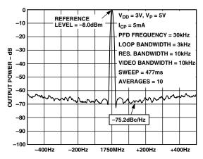
TPC 10. ADF4213 Phase Noise (1750 MHz, 30 kHz, 3 kHz)
