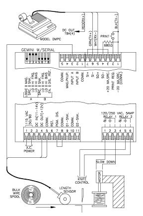
This application depicts a GEMINI 2000 controlling a coil winding machine. A length sensor provides output units in feet. Output 1 is used as the slow-down for the drive motor and Output 2 is used for the cut off knife control. A printer is used to record the length of each coil that is wound. Preset 1 is set to the slow down length and Preset 2 is set to the desired length of the coil.
