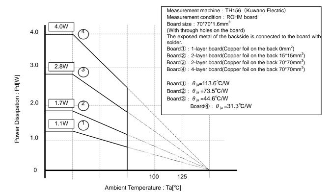
Fig.2 HTSSOP-B24 Derating curve
