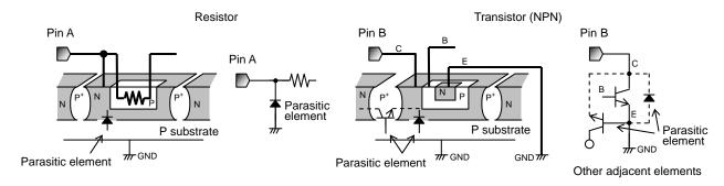
Fig.3 Pattern Diagram of Parasitic Element
