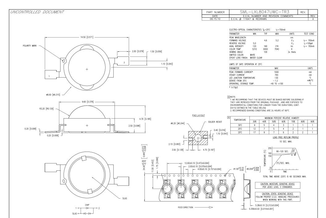
\*UNLESS OTHERWISE SPECIFIED TOLERANCES PER DECIMAL PRECISION ARE: X=±1 (±0.039), X.X=±0.5 (±0.020), X.XX=±0.25 (±0.010), X.XXX=±0.127 (±0.005). LEAD SIZE=±0.05 (±0.002), LEAD LENGTH=±0.75 (±0.030). MIN= +DECIMAL PRECISION MAX.= +0.00 -DECIMAL PRECISION PRECISION PRECISION MAX.= +0.00 -DECIMAL PRECISION PRECISION PRECISION MAX.= +0.00 -DECIMAL PRECISION PRECISION PRECISION PRECISION MAX.= +0.00 -DECIMAL PRECISION PRECISION PRECISION PRECISION MAX.= +0.00 -DECIMAL PRECISION PRECISION
