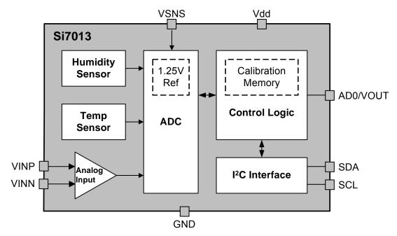
Figure 8. Si7013 Block Diagram
