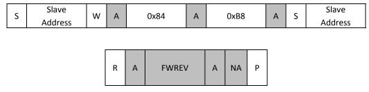
The upper nibble of the FWREV byte corresponds to the major firmware revision number, while the lower nibble of the FWREV byte corresponds to the minor firmware revision number. Therefore, firmware revision 1.0 would be encoded as 0x10 in the FWREV byte.
