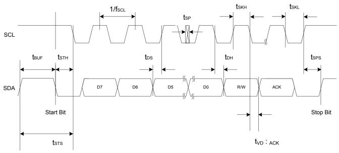
Figure 1. I<sup>2</sup>C Interface Timing Diagram
