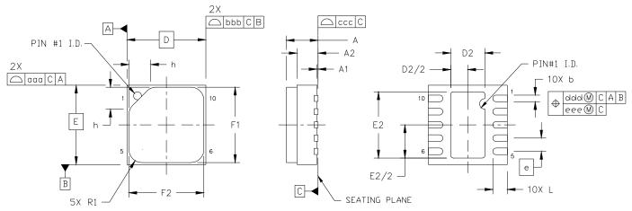
Figure 12. 10-pin DFN with Protective Cover
