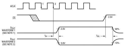
**NOTE 1:** WAVEFORM 1 IS FOR AN OUTPUT WITH INTERNAL CONDITIONS SUCH THAT THE OUTPUT IS HIGH UNLESS DISABLED BY THE OUTPUT CONTROL.
