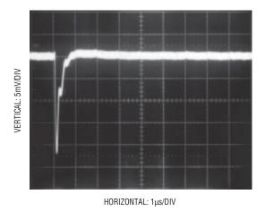
Figure 11. Adequate Settling of Op Amp Driving Analog Input
