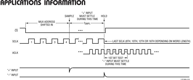
Figure 10. "+" and "-" Input Settling Windows
