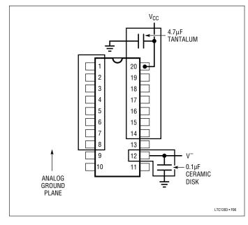
Figure 6. Example Ground Plane for the LTC1283
