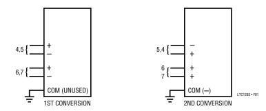
Figure 1. Examples of Multiplexer Options on the LTC1283
