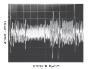
Figure 7. Poor V<sub>CC</sub> Bypassing. Noise and Ripple can Cause A/D Errors
