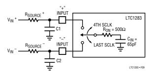
Figure 9. Analog Input Equivalent Circuit
