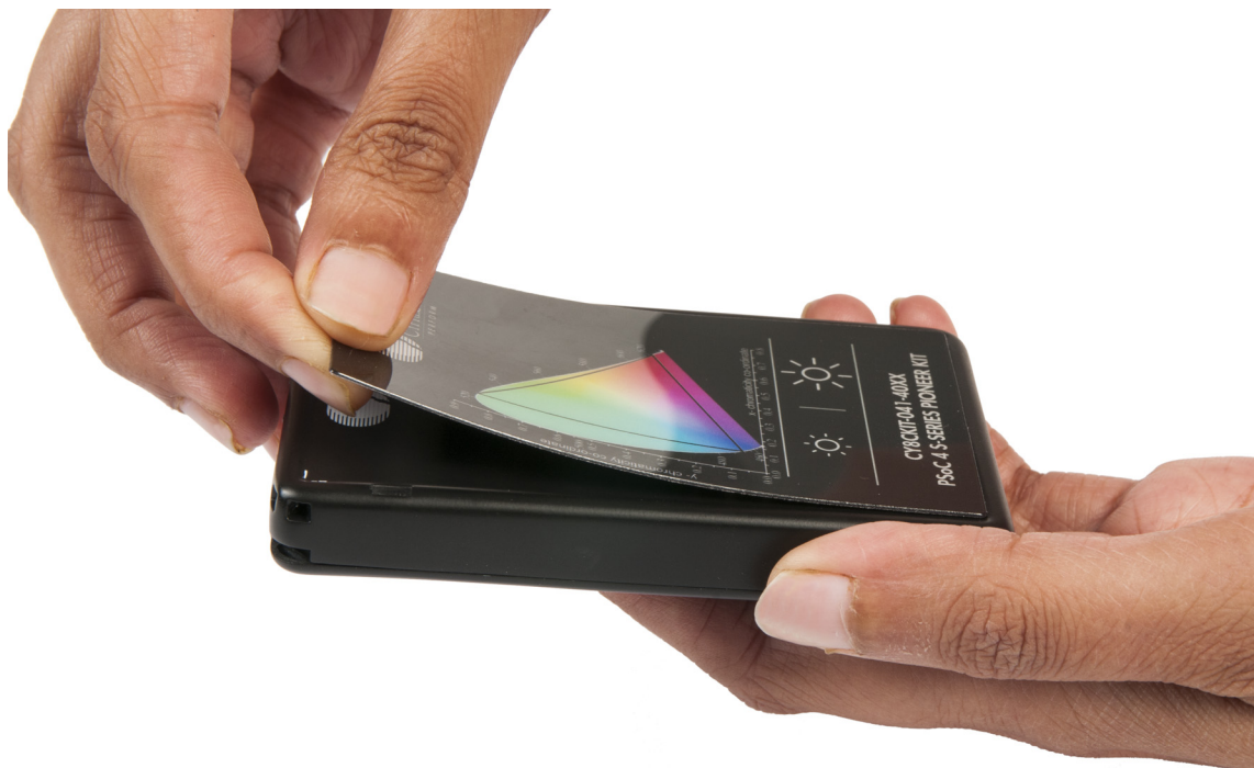
Figure 3-10. Removing the Overlay
