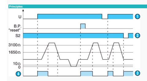
The relay is reset either using the RESET pushbutton on the front face or by opening the external contact S2 (remote reset), or by cutting the auxiliary power supply (terminals A1 - A2). If the auxiliary power is cut for a period of time greater than the reset time (500 ms), the relay is reactivated if the proble detects a normal temperature when the power supply voltage is restored.
