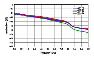
**Figure 3. Insertion Loss vs Frequency**
