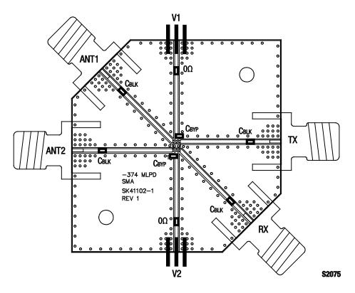
Figure 8. SKY13381-374LF Evaluation Board Assembly Diagram
