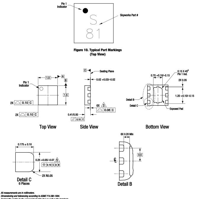
Coplanarity applies to the exposed heat sink slug as well as the terminals ..
