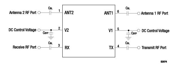
Figure 7. SKY13381-374LF Evaluation Board Schematic
