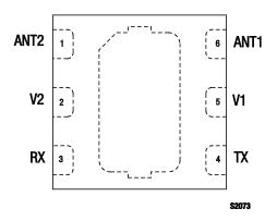
Figure 2. SKY13381-374LF Pinout – 6-Pin MLPD (Top View)
