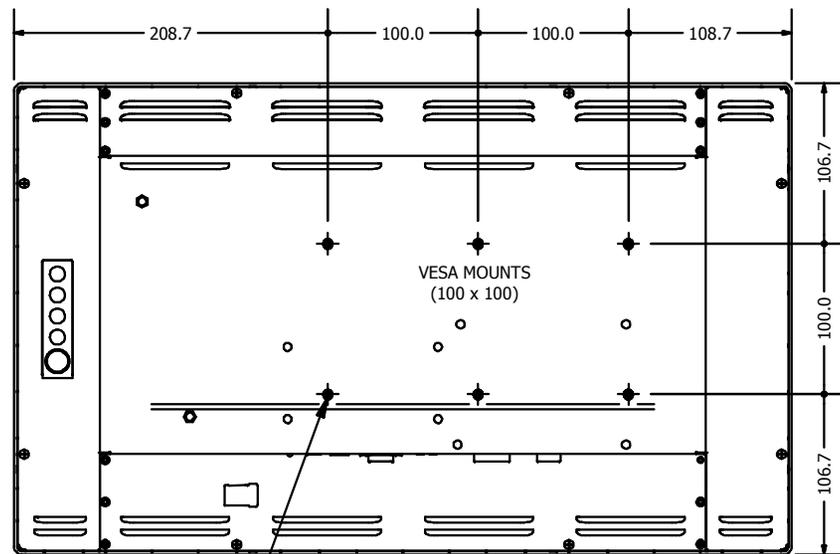
The distance between the back cover surface and the bottom of the screw hole is 8 mm. Please use four M4 screws with the proper length to mount the monitor if you are not using the included mounting brackets and M4x6 screws.
