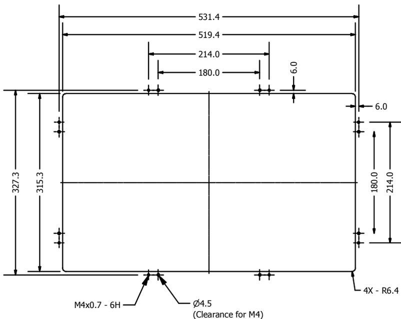
1. Inside two holes (180 mm) for M4 clearance holes.
