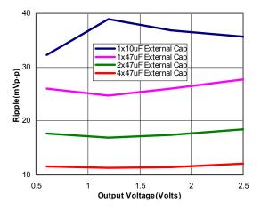
Figure 37. Output ripple voltage for various output voltages with external 1x10  $\mu$ F, 1x47  $\mu$ F, 2x47  $\mu$ F or 4x47  $\mu$ F ceramic capacitors at the output (20A load). Input voltage is 3.3V.
