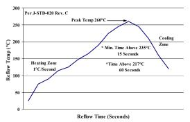
Figure 47. Recommended linear reflow profile using Sn/Ag/Cu solder.
