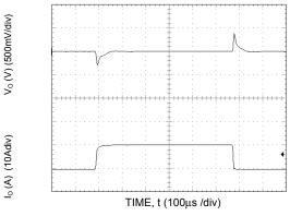
Figure 28. Transient Response to Dynamic Load Change from 0% 50% to 0% with V\_IN=5V.
