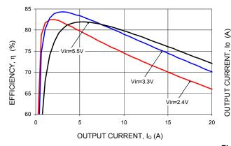
The following figures provide typical characteristics for the TLynx<sup>™</sup> at 0.6Vo and at 25°C.
