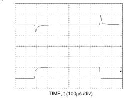
Figure 10. Transient Response to Dynamic Load Change from 0% to 50% to 0% with  $V_{IN}$ =3.3V.
