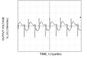
Figure 15. Typical output ripple and noise (VIN = 3.3V,  $I_0 = I_{0,max}$ ).
