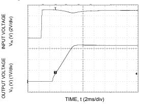
Figure 30. Typical Start-up Using Input Voltage (VIN = 5V,  $I_0 = I_{0,max}$ ).
