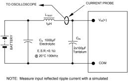
OTE: Measure input reflected npple current with a simulated source inductance (L<sub>TEST</sub>) of 1µH. Capacitor C<sub>S</sub> offsets possible battery impedance. Measure current as shown above.
