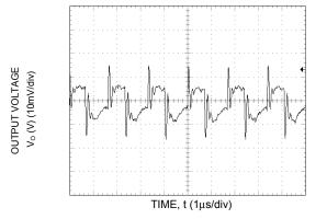
Figure 9. Typical output ripple and noise (VIN = 3.3V,  $I_0 = I_{0,max}$ ).
