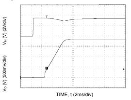
Figure 18. Typical Start-up Using Input Voltage (VIN = 3.3V, Io = Io,max).
