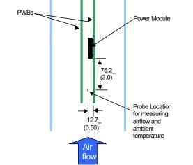
Figure 45. Thermal Test Setup.
