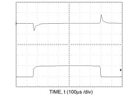
Figure 16. Transient Response to Dynamic Load Change from 0% to 50% to 0% with  $V_{IN}$ =3.3V.
