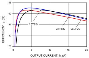
The following figures provide typical characteristics for the TLynx<sup>™</sup> at 1.8Vo and at 25°C.
