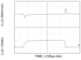
Figure 4. Transient Response to Dynamic Load Change from 0% to 50% to 0% with  $V_{\text{IN}}\text{=}3.3V.$
