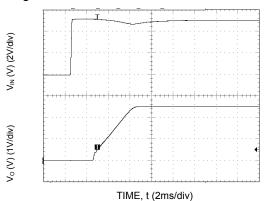
Figure 24. Typical Start-up Using Input Voltage (VIN = 5V,  $I_0 = I_{0,max}$ ).
