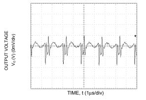
Figure 21. Typical output ripple and noise (VIN = 3.3V, Io = Io,max).
