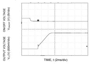
Figure 11. Typical Start-up Using On/Off Voltage ( $I_0 = I_{0,max}$ ).
