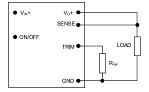
Figure 41. Circuit configuration for programming output voltage using an external resistor.
