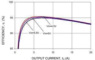
The following figures provide typical characteristics for the TLynx<sup>™</sup> at 3.3Vo and at 25°C.
