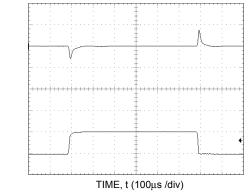
Figure 22. Transient Response to Dynamic Load Change from 0% to 50% to 0% with  $V_{IN}$ =5V.
