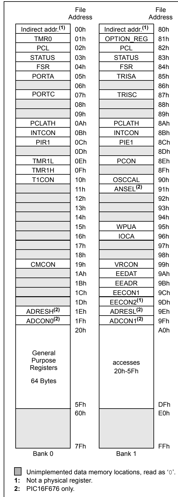
FIGURE 2-2: DATA MEMORY MAP OF THE PIC16F630/676
