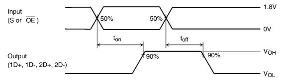
Fig. 11.2 Turn-ON and Turn-OFF Times (ton, toff)
