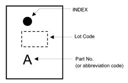
Fig. 5.1 Marking (Top view)
