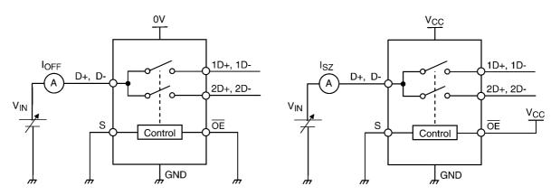
Fig. 11.10 Power-OFF Leakage Current
