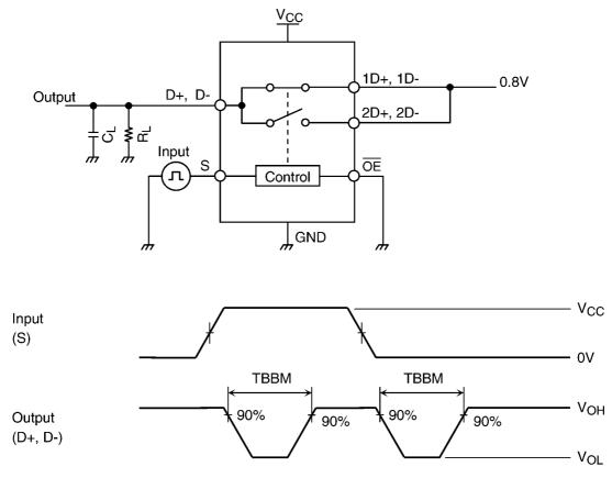
Fig. 11.3 Break Before Make (TBBM)
