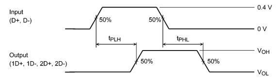
Fig. 11.1 Propagation Delay Time (t<sub>PLH</sub>, t<sub>PHL</sub>)
