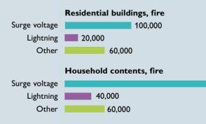
Device failure or defects caused by surge voltages are more frequent than expected. According to the statistics of the German Insurance Association (GDV), surge voltages are the most common cause of damage. These figures only apply to damage that resulted in fire.
