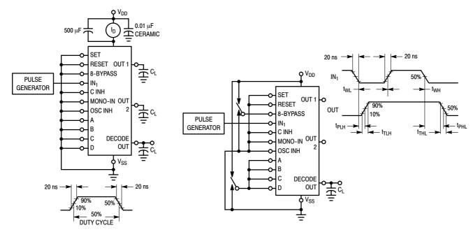
Figure 8. Power Dissipation Test Circuit and Waveform
