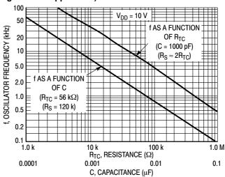
Figure 3. RC Oscillator Stability
