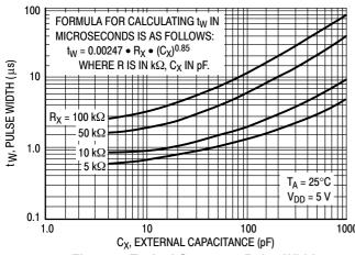
Figure 5. Typical C<sub>X</sub> versus Pulse Width @ V<sub>DD</sub> = 5.0 V
