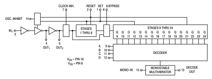
Figure 2. Block Diagram
