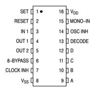
Figure 1. Pin Assignment
