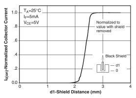
Figure 2. Normalized Collector Current Vs. Shield Distance
