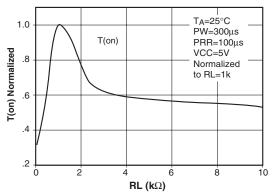
Figure 6. Fall Time vs. Load Resistance
