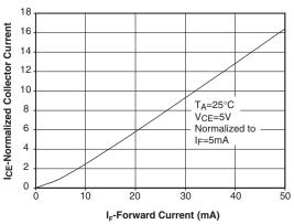
Figure 4. Normalized Collector Current Vs. Forward Current
