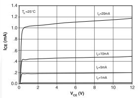
Figure 3. Collector Current Vs. Collector-Emitter Voltage
