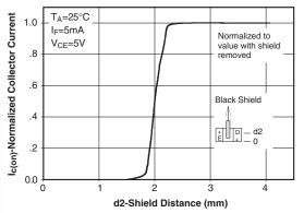
Figure 1. Normalized Collector Current Vs. Shield Distance
