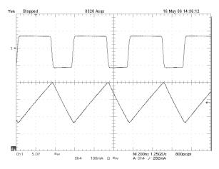
Figure 9. Continuous Conduction Mode (CCM) 1 SWN, 5 V/div DC, 4 I<sub>LN</sub>, 100 mA/div, DC, I<sub>OUTN</sub> = 100 mA
