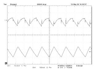
Figure 11. Positive Output Voltage Ripple in CCM 1  $V_{OUTP}$ , 10 mV/div AC, 4 I<sub>LP</sub>, 100 mA/div DC, I<sub>OUTP</sub> = 100 mA
