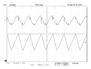
Figure 12. Negative Output Voltage Ripple in CCM 1  $V_{OUTN}$ , 10 mV/div AC, 4 I<sub>LN</sub>, 100 mA/div DC, I<sub>OUTN</sub> = 100 mA
