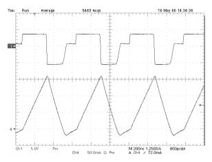
Figure 10. Discontinuous Current Mode (DCM) 1 SWN, 5 V/div, DC 4 I<sub>LN</sub>, 50 mA/div, DC, I<sub>OUTN</sub> = 20 mA
