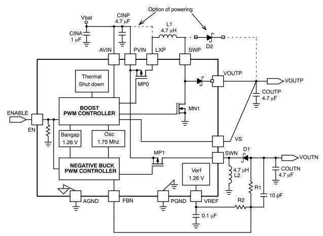
Figure 2. Simplified Block Diagram
