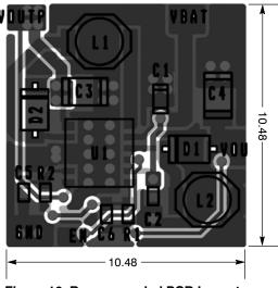
Figure 16. Recommended PCB Layout
