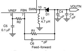
Figure 15. Inverter Compensation
