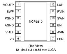
Exposed pad must be soldered to PCB Ground plane
