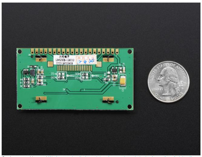
Getting started is easy! We have a detailed tutorial and example code in the form of an Arduino library for text and graphics. (http://adafru.it/j6a) You'll need a microcontroller with more than 512 bytes of RAM since the display must be buffered. The library can print text, bitmaps, pixels, rectangles, circles and lines. It uses 512 bytes of RAM since it needs to buffer the entire display but its very fast! The code is simple to adapt to any other microcontroller.
