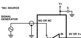
Signal direction through switch is reversed, worst case values are recorded. Repeat test for all switches.
