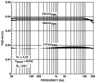
FIGURE 20. TOTAL HARMONIC DISTORTION vs FREQUENCY
