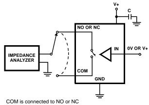
during ON capacitance measurement.
