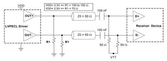
Figure 4. LVPECL AC Coupled Termination
