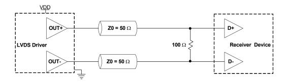
Figure 6. LVDS Single Termination (Load Terminated)
