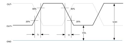
Figure 1(a). LVPECL Voltage Levels per Differential Pin (OUT+/OUT-)
