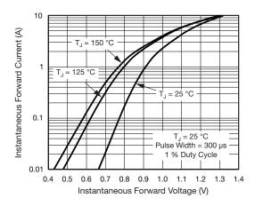
Fig. 3 - Typical Forward Voltage Characteristics Per Diode
