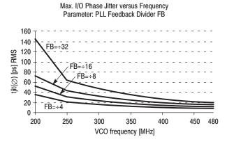
Figure 9. MPC9772 I/O Jitter
