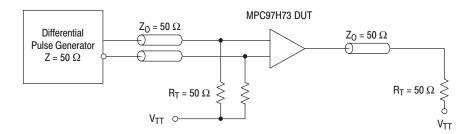
Figure 16. PCLK MPC97H73 AC test reference
