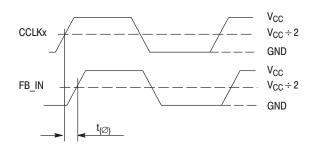
Figure 18. Propagation delay  $(\mathbf{t}_{(\emptyset)},$  static phase offset) test reference
