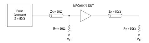
Figure 15. CCLK MPC97H73 AC test reference
