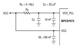
Figure 7. V<sub>CC\_PLL</sub> Power Supply Filter
