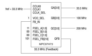
MPC97H73 example configuration (feedback of QFB = 33.3 MHz,  $f_{VCO}$ =400 MHz,  $VCO\_SEL$ = $\div$ 1, M=12,  $N_A$ =12,  $N_B$ =4,  $N_C$ =2).
