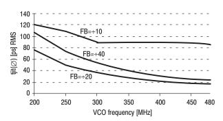
Figure 11. MPC9772 I/O Jitter
