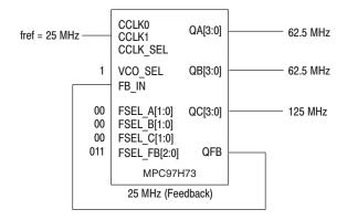
MPC97H73 example configuration (feedback of QFB = 25 MHz,  $f_{VCO}$ =250 MHz, VCO\_SEL= $\div$ 1, M=10, N<sub>A</sub>=4, N<sub>B</sub>=4, N<sub>C</sub>=2).
