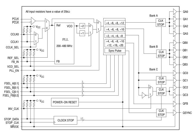
Figure 1. MPC97H73 Logic Diagram
