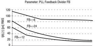
Max. I/O Phase Jitter versus Frequency
