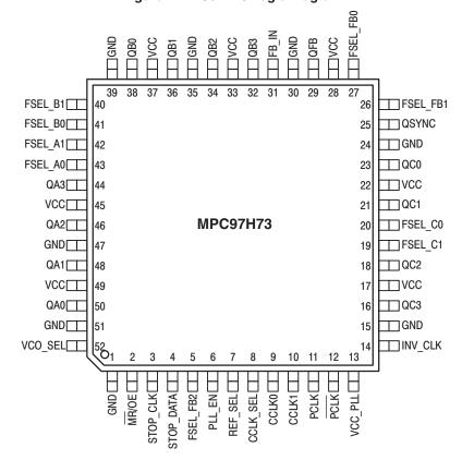
Figure 2. MPC97H73 52-Lead Package Pinout (Top View)
