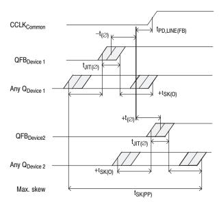
Figure 8. MPC97H73 max. device-to-device skew
