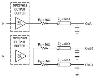
Figure 12. Single versus Dual Transmission Lines
