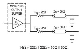
$25\Omega = 25\Omega$  Figure 14. Optimized Dual Line Termination
