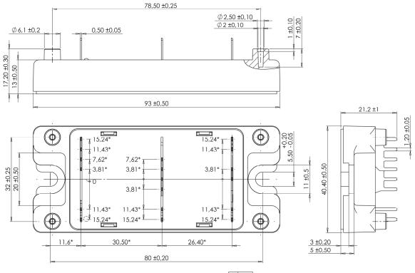
ALL DIMENSIONS MARKED "\*" ARE TOLERANCED AS : + Ø 1
