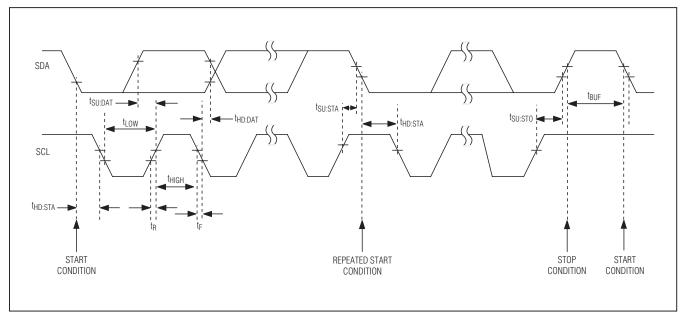
Figure 1. SMBus Timing Diagram
