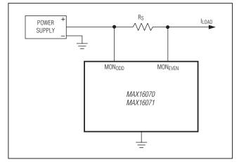
Figure 16. Current Monitoring Connection
