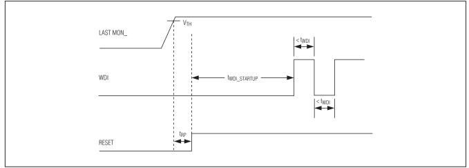
Figure 5. Normal Watchdog Startup Sequence
