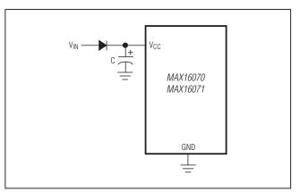
Figure 14. Power Circuit for Shutdown During Fault Conditions
