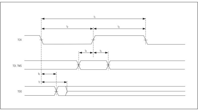
Figure 2. JTAG Timing Diagram
