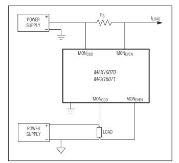
Figure 3. Differential Measurement Connections
