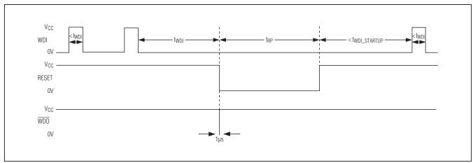
Figure 7. Watchdog Startup Sequence with Watchdog Reset Output Enable Bit Set to '1'
