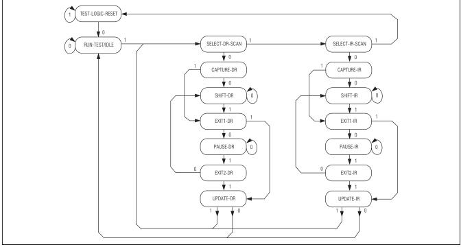
Figure 13. Tap Controller State Diagram
