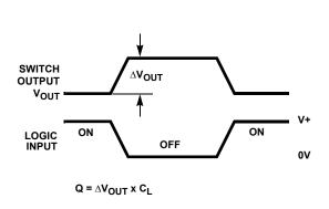
FIGURE 2A. MEASUREMENT POINTS
