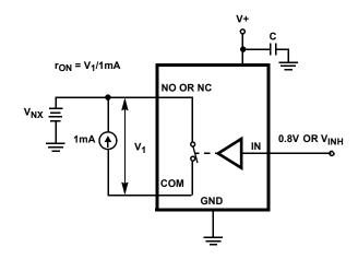
FIGURE 5. ron TEST CIRCUIT
