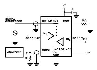
FIGURE 6. CROSSTALK TEST CIRCUIT
