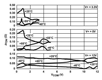
FIGURE 11. ron MATCH vs SWITCH VOLTAGE
