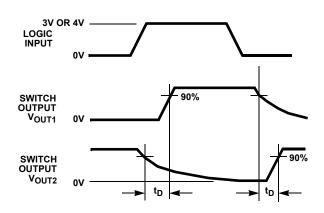
FIGURE 3A. MEASUREMENT POINTS (ISL43122 ONLY)
