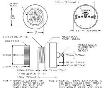
NOTE A: TERMINALS—032 BRASS TIN PLATED, TAPPED FUR #6-32 SCREW. TWO #6-32 NICKEL PLATED BRASS SCREWS INCLUBED. WILL ACCEPT 1/4" QUICK CONNECT.
