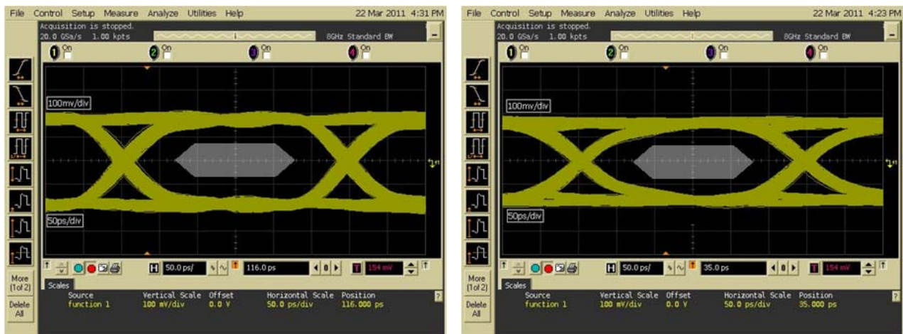
Figure 10. EMI4163MU Measured Eye Diagram @ 3.4Gbps (EVB through on left, EVB with EMI4163MU on right)
