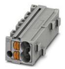
Marshalling patchboard, Nom. voltage: 500 V, Nominal current: 17.5 A, Cross section: 0.14 mm² - 2.5 mm², AWG: 12 - 26, Connection type: Push-in connection, Number of positions: 1, Number of connections: 4, Width: 11 mm, Length: 8.6 mm, Color: gray, Color of connection elements: brown, Assembly: for snapping onto a DIN rail adapter, for snapping onto a cover flange
