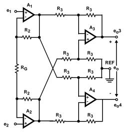
FIGURE 30. DIFFERENTIAL OUTPUT AMPLIFIER
