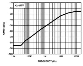
FIGURE 17. COMMON-MODE REJECTION RATIO (CMRR)
