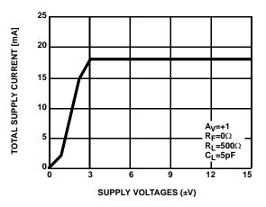
FIGURE 25. SUPPLY CURRENT vs SUPPLY VOLTAGE
