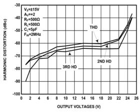
FIGURE 20. HARMONIC DISTORTION vs OUTPUT VOLTAGE  $(A_V = +2)$
