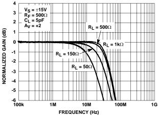
FIGURE 10. GAIN vs FREQUENCY FOR VARIOUS  $R_{LOAD}$ (A<sub>V</sub> = +2)
