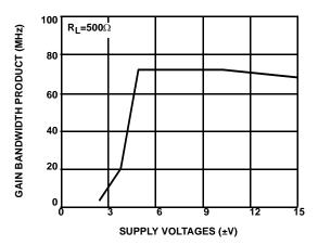
FIGURE 7. GAIN BANDWIDTH PRODUCT vs SUPPLY
