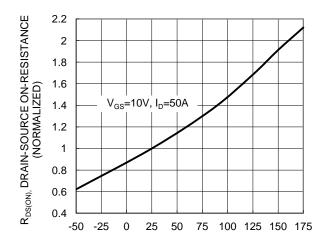
T<sub>J</sub>, JUNCTION TEMPERATURE (°C) Figure 6. On-Resistance Variation with Temperature
