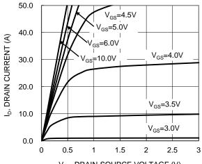
V<sub>DS</sub>, DRAIN-SOURCE VOLTAGE (V) Figure 1. Typical Output Characteristic
