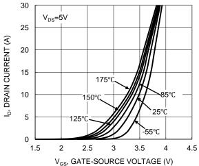
Figure 2. Typical Transfer Characteristic
