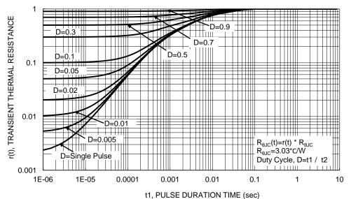
Figure 13. Transient Thermal Resistance
