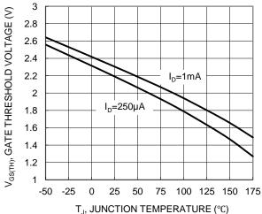
Figure 8. Gate Threshold Variation vs Temperature
