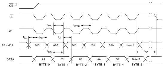
Notes: 1.  $\overline{OE}$  must be high only when  $\overline{WE}$  and  $\overline{CE}$  are both low.
