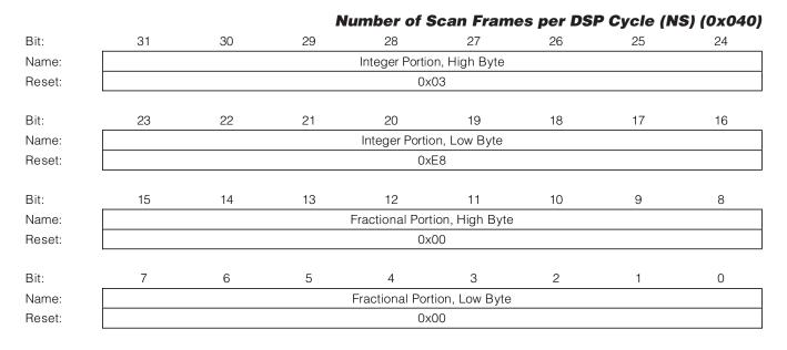
The NS register defines the fundamental timing for the electricity meter. It defines a DSP cycle in terms the period of the ADC scan frame. Generally, this register is calculated and updated automatically by the MAXQ3181 firmware based on the zero-crossing detection, and whether noise rejection (REJ\_NS) and averaging (AVG\_NS) are enabled. Host code can write to this register in order to set the desired DSP cycle duration. The duration of one scan frame (tFR) is represented as 0x00010000.
