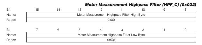
This register specifies the b<sub>0</sub> coefficient of a first-order Butterworth filter using the following formula:
