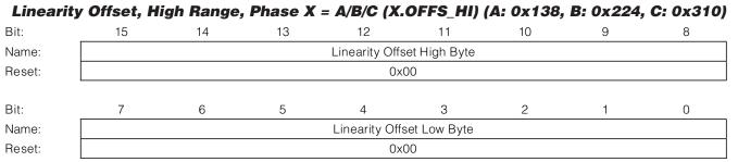
This signed register contains the linearity offset for phase X current channel when the programmable gain amplifier is set to unity gain (that is, the measured current is above the low current threshold). The signed value represented by this register is added to the current value according to following formula:
