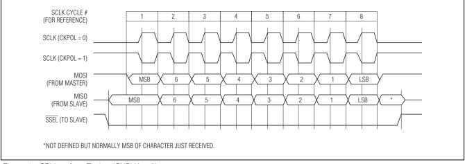
Figure 4a. SPI Interface Timing (CKPHA = 0)
