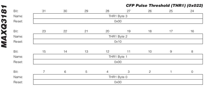
This register designates the threshold of the CFP pulse. This value is used to set the meter constant for the CFP pulse output. When the CFP pulse accumulator exceeds the value set in this register, the CFP pulse output is activated and the CFP pulse accumulator is reduced by the amount in this register.
