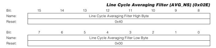
This register determines whether the NS value is averaged over previous values or whether the most recently measured value is used directly. If the value of this register is nonzero, the NS value is averaged using the following formula:
