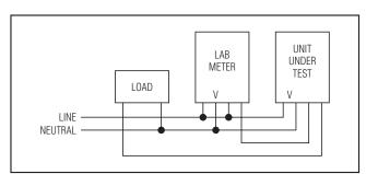
Figure 15. Offset Testing Setup
