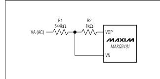
Figure 13. Sample Voltage Input Circuit
