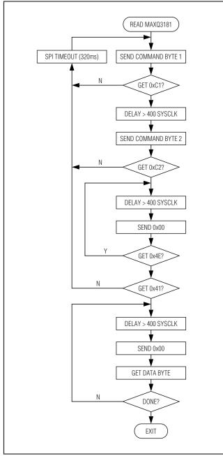
Figure 7. Flowchart for Reading from MAXQ3181
