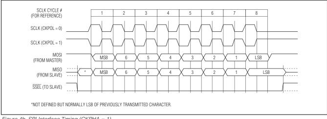
Figure 4b. SPI Interface Timing (CKPHA = 1)
