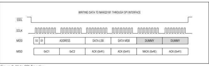
Figure 6. Write SPI Transfer
