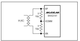
Figure 14. Sample Current Input Circuit
