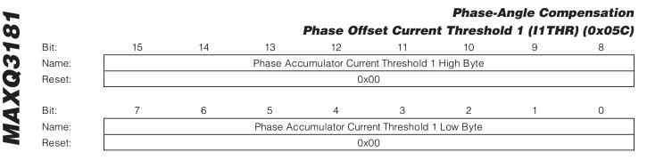
This register specifies the fraction of full-scale current that causes the MAXQ3181 to switch from PA0 to PA1 to provide phase-angle compensation. For more information, see the PA0, PA1, and PA2 register descriptions. The full-scale current is represented by 0x10000.
