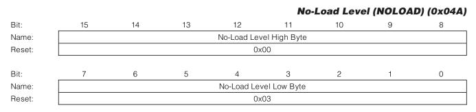
This register specifies the fraction of full-scale current below which a no-load condition is declared. When X.IRMS falls below this level, the MAXQ3181 no longer accumulates power for phase X. Full scale is represented by 0x10000. The maximum value for this register is 0xFFFF.
