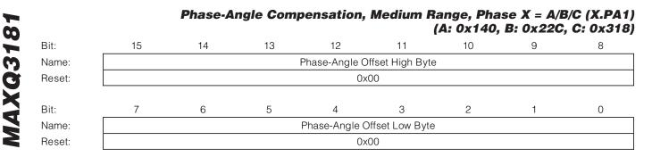
This signed register contains the angle, as a fraction of one radian, to add to the measured phase angle when the measured current is between the values given in I1THR and I2THR. This signed value ranges from -0.5 radian (at a value of 0x8000) to  $+(0.5 - 2^{-16})$  radian (at a value of 0x7FFF).
