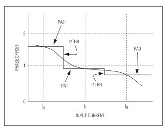
Figure 16. Phase Offset vs. Input Current Calibration
