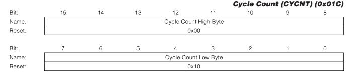
This register contains the number of line cycles that will be accumulated in a single DSP cycle. When CYCNT line cycles have been accumulated, the DSP performs power, power factor, and energy calculations. By default, the cycle count is 0x10 (16 decimal).
