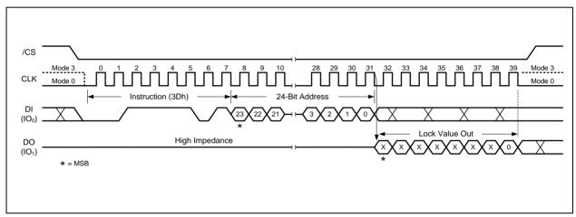
Figure 53a. Read Block Lock Instruction (SPI Mode)
