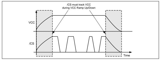
Figure 57b. Power-up, Power-Down Requirement
