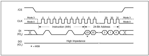
Figure 44. Erase Security Registers Instruction (SPI Mode only)
