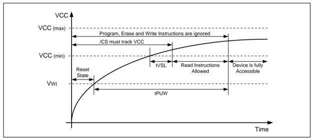
Figure 57a. Power-up Timing and Voltage Levels
