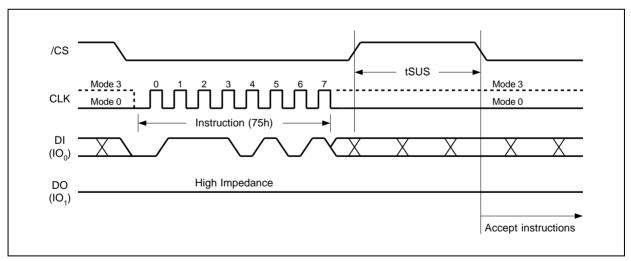
Figure 35a. Erase/Program Suspend Instruction (SPI Mode)
