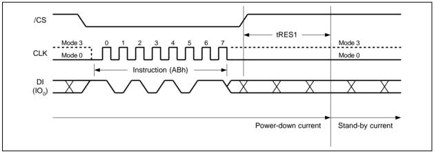
Figure 38a. Release Power-down Instruction (SPI Mode)
