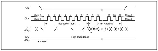
Figure 52a. Individual Block Unlock Instruction (SPI Mode)
