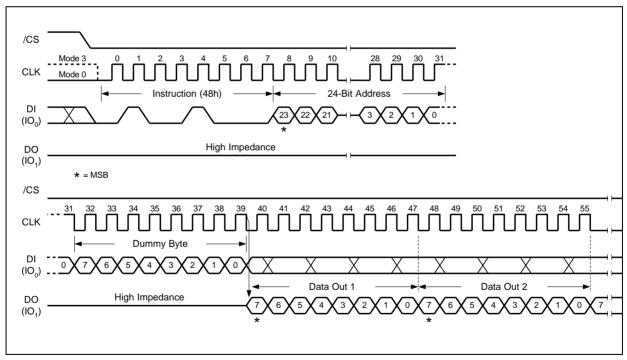
Figure 46. Read Security Registers Instruction (SPI Mode only)
