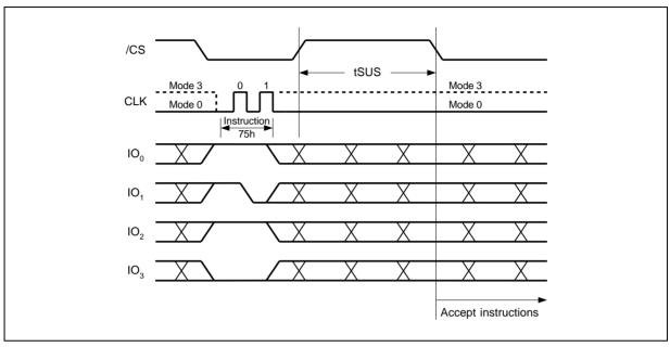
Figure 35b. Erase/Program Suspend Instruction (QPI Mode)
