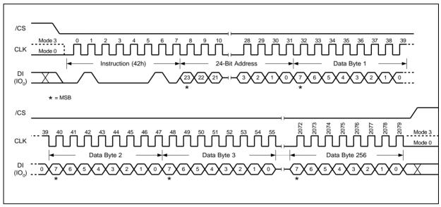
Figure 45. Program Security Registers Instruction (SPI Mode only)
