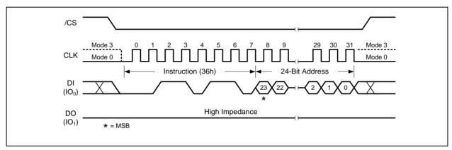
Figure 51a. Individual Block/Sector Lock Instruction (SPI Mode)
