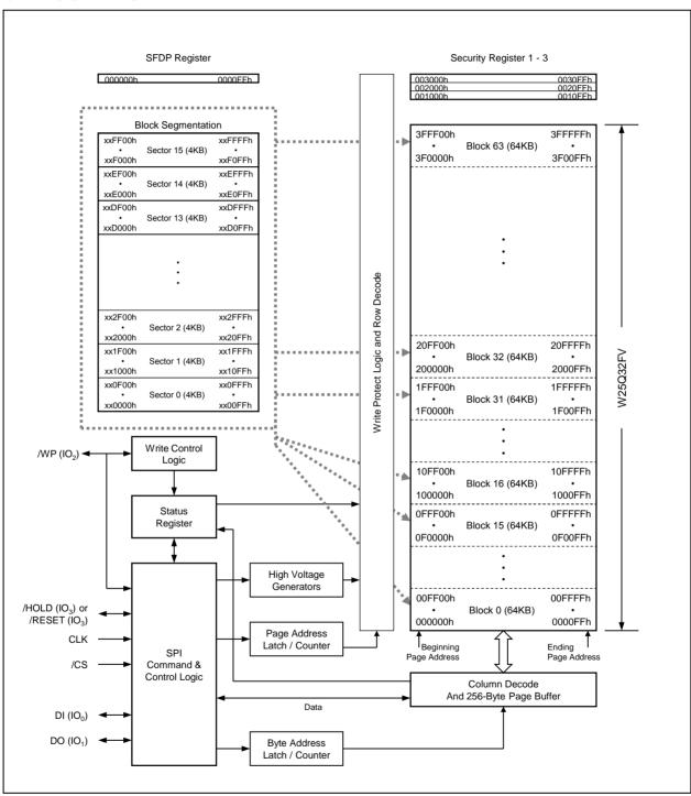
Figure 2. W25Q32FW Serial Flash Memory Block Diagram
