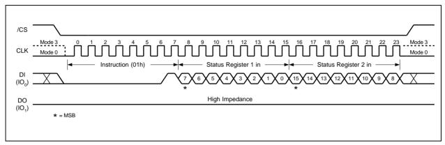
Figure 9c. Write Status Register-1/2 Instruction (SPI Mode)
