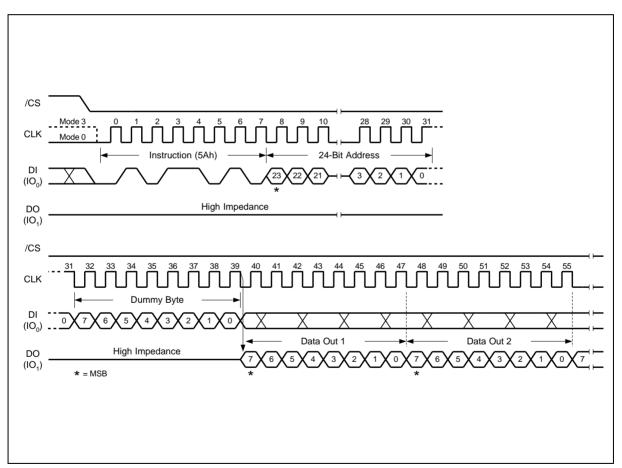
Figure 34. Read SFDP Register Instruction Sequence Diagram
