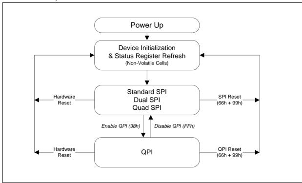
Figure 3, W25Q32FW Serial Flash Memory Operation Diagram
