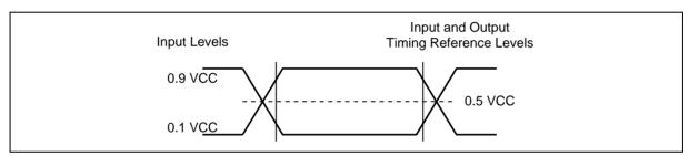
Figure 58. AC Measurement I/O Waveform
