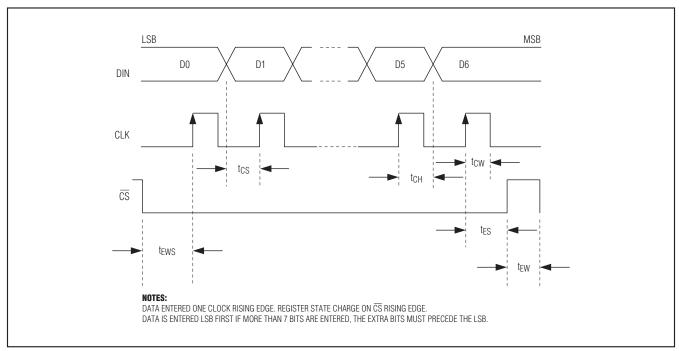
Figure 1. Shift Register Timing Diagram
