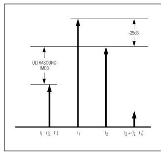
Figure 2. Ultrasound IMD3 Measurement Technique
