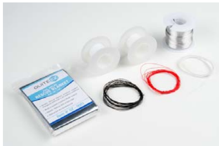
Two small empty wire spools (or plastic cups), 16 AWG jewelry wire, emergency blanket, 30 AWG wire wrapping wire.
