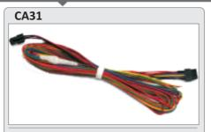
Main port extended installation cable with an 8pin double row, UCOM connector and open ends. Open wires (6pin): 3 x IOs, IGN, V+, GND
