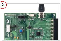
Ensure that shunt is placed between 5 V and VCC of jumper J1. Plug in the USB cable to the CY3280-20x66 Universal CapSense Controller Board.
