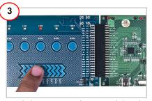
Touch the CapSense button or slider. The respective LEDs lights up.
