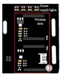
Two wireless slots available which allow Xbee, blusteeth/Wifi to be used at the same time.
