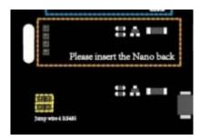
There are 2 Nano slots on the GMR. For general mobile robot, this two micro controllers can help you to solve the motor control and driver some special sensors. And they all have connected with the main micro controller Mega ADK or Mega 2560. The communication way is the I2C.
