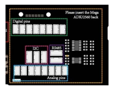
The main controller of this GMR board. Because of the high performance of the Arduino Mega ADK/2560. For the GMR, 8 I/O and 8 analog pins can be used. 3 groups of I2C pins can communicated with other controllers and 2 groups of RS485 belongs to another nano controller.
