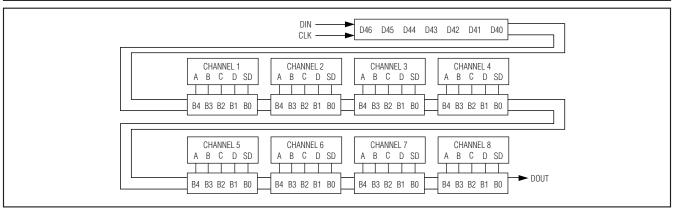
Figure 1. Data Flow of Serial Shift Register
