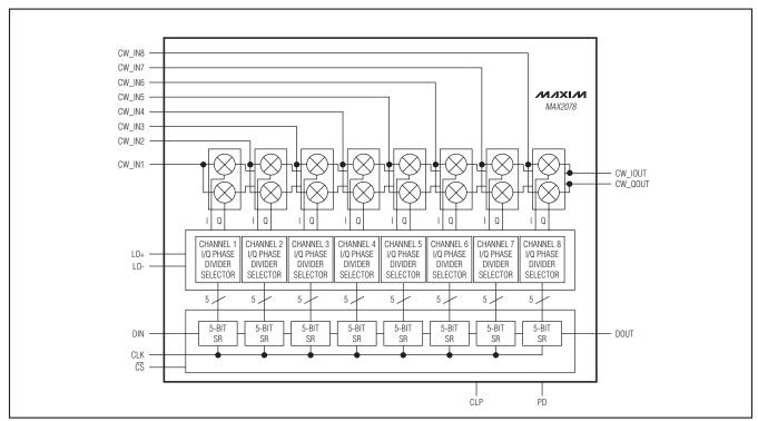
Each mixer can be programmed to 1 of 16 phases; therefore, 4 bits are required for each channel for programming. Each CW channel can be programmed to an off state by setting bit Di to 1. The power-down mode (PD) line overrides this soft shutdown.
