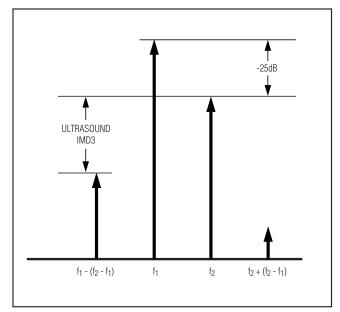
Figure 6. Ultrasound IMD3 Measurement Technique
