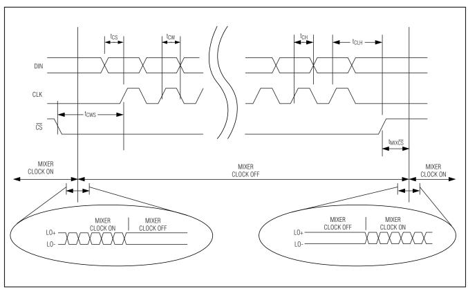
Figure 5. Shift Register Timing Diagram
