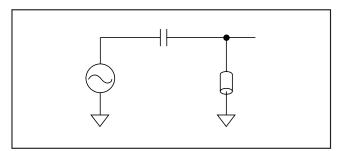
Figure 3. Simplified Circuit of Highpass Pole
