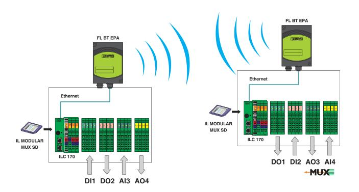
The software on the SD FLASH 512MB MODULAR MUX CompactFlash® card transforms the ILC 131 ETH and the individual input and output terminals required into a flexible field multiplexer. As a wireless connection or as a point-to-point connection in an Ethernet network.
