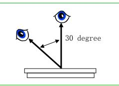
Under daylight lamp 20 $\sim40W_{\rm F}$  product distance inspector'eye 30cm,incline degree 30°  $_{\circ}$
