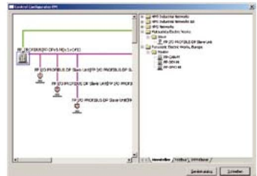
Control Configurator FM is an add-on software for Control FPWIN Pro and is used to configure and diagnose the FMUs. Part number: AFPS35510
