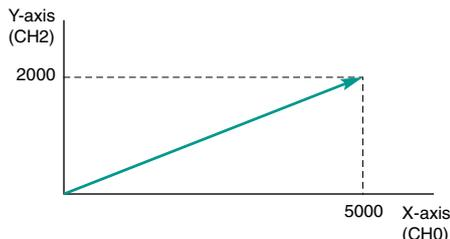
A control function that automatically defines the continuum of points in a straight line based on only two coordinate positions.
