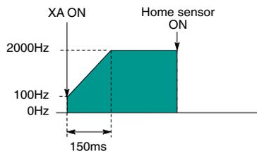
Home search automatically reverses the motor rotation when Over limit input(+) or Over limit input (-) is input and their searches for the home position or near home position in order to return to it automatically.
