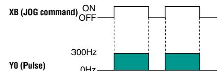
This refers to an operation in which the motor is rotated only while operation commands are being input. This is used to forcibly rotate the motor using input from an external switch, for instance when making adjustments. Depending on the circumstances, unlimited feeding can be accomplished with the JOG operation in some cases.
