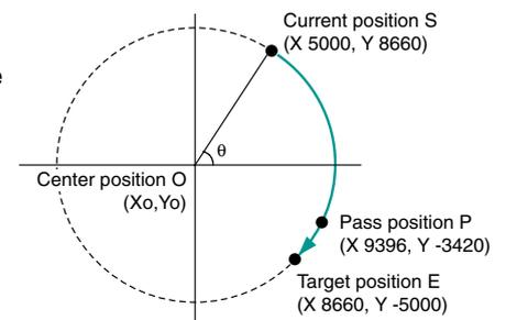
Allows points to be smoothly traversed by arced paths for which the user specifies the orientation plane, the radius of curvature, motion path profile and direction of motion.
