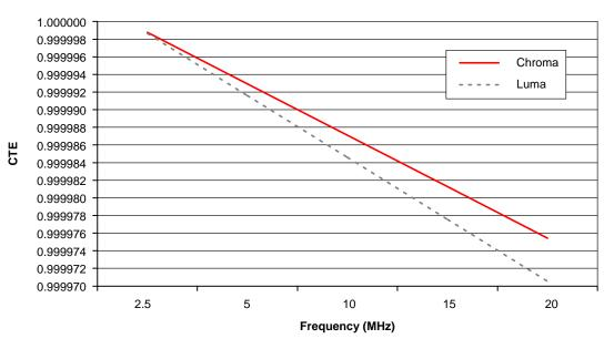
Figure 17. CTE vs. Frequency
