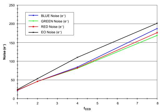
Typical KLI–2104 Dark Noise vs. CCD Clock Frequency
