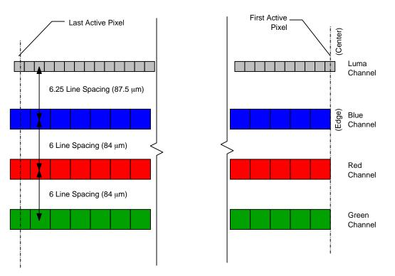
Figure 4. Active Pixel and Channel Alignment - KLI-2104
