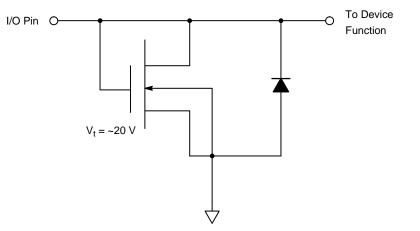
**CAUTION:** To allow for maximum performance, this device was designed with limited input protection; thus, it is sensitive to electrostatic induced damage. These devices should be installed in accordance with strict ESD handling procedures!
