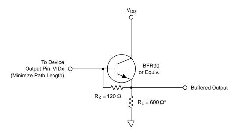
Figure 23. Typical Output Bias/Buffer Circuit
