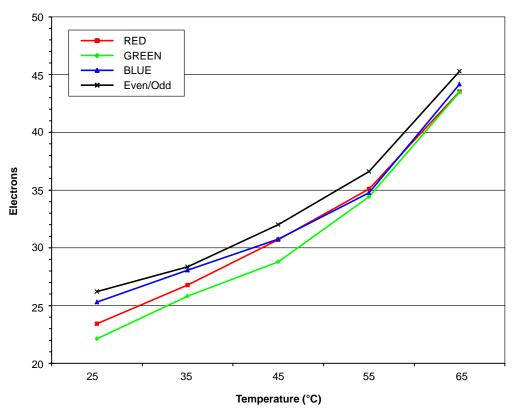
Figure 14. Dark Noise vs. Temperature
