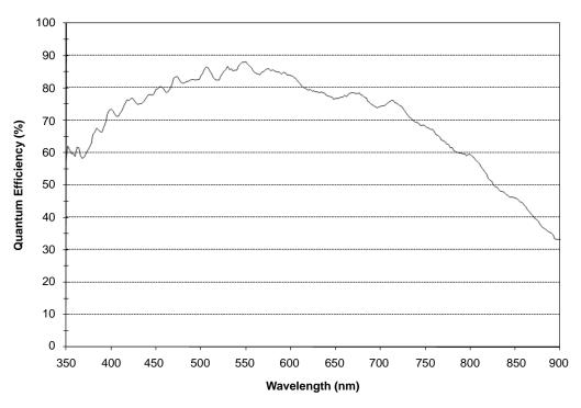
KLI-2104 Quantum Efficiency – Even/Odd Monochrome Channels
