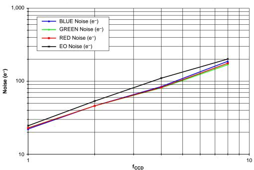
Typical KLI-2104 Dark Noise vs. CCD Clock Frequency
