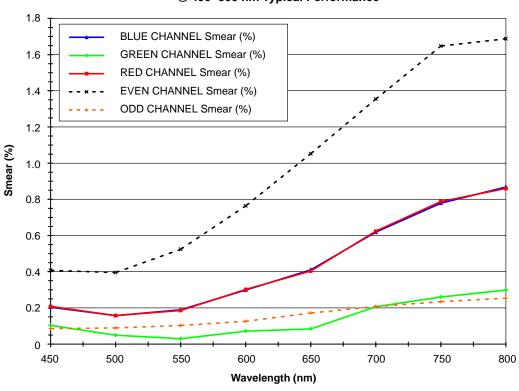
KLI-2104 Smear (Photodiode-to-CCD Crosstalk) @ 450-800 nm Typical Performance
