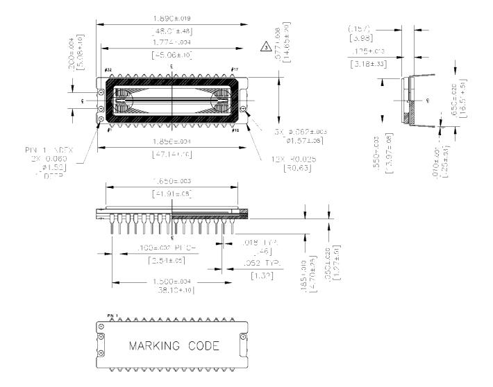
Figure 26. Completed Assembly
