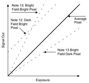
Figure 6. Defective Pixel Classification
