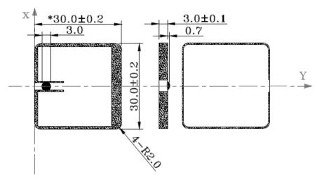
Mounting: The antenna is mounted with double sided adhesive tape that is attached to the underside of the antenna.
