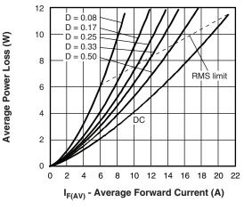
Fig. 6 - Forward Power Loss Characteristics
