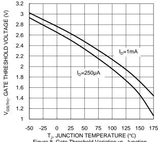
T<sub>J</sub>, JUNCTION TEMPERATURE (°C) Figure 8. Gate Threshold Variation vs. Junction Temperature
