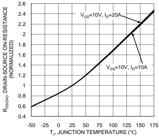
Figure 6. On-Resistance Variation with Temperature
