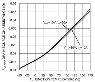
Figure 7. On-Resistance Variation with Temperature
